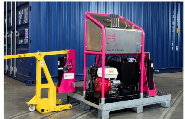
**Capacity up to 40ft/32 tonnes - TÜV/CE marked - Simple 2 man operation - Colour coded hoses - Easy storage & handling - Patent Pending - Container weighing - Removes need for craneage**
